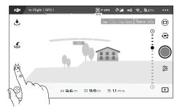
3. Tap on the subject you want to track then tap to confirm your selection. If the subject is not automatically recognized, drag a box around it. The box will turn green when tracking is in progress. If the box turns red, the object could not be identified and you should try again.
