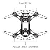
The Front LEDs show the orientation of the aircraft and the status of some functions (please refer to the Gesture Mode "Feature Descriptions" section for more details). The Front LEDs glow solid red when the aircraft is turned on to indicate the front or nose of the aircraft.
