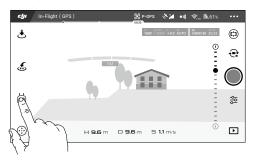
3. Tap once on the target and wait for the "GO" icon to appear. Tap the "GO" icon to confirm the selection and the aircraft will fly to the target automatically. There will be a prompt if the target cannot be reached. If this is the case, select another target and try again.
