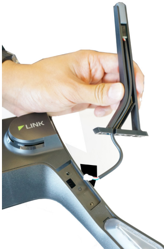
Figure 10.4.3.2: Insert New Leg with Compass
