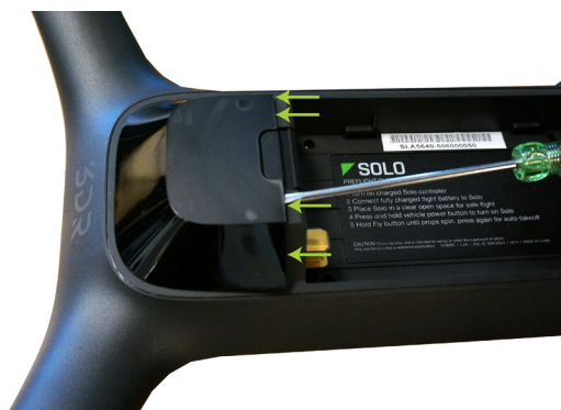
Figure 10.5.1.1: GPS Cover Removal
