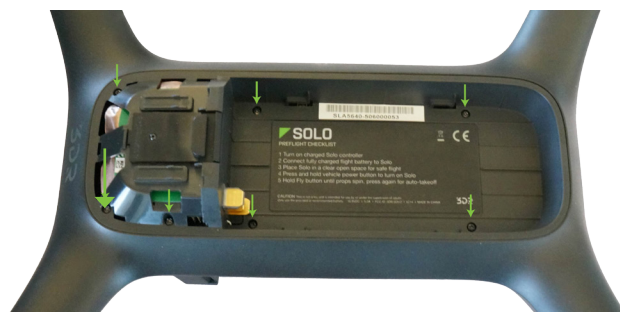
Figure 10.5.2.1: Battery Tray Removal
