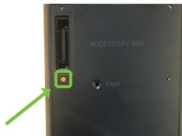
Figure 10.7.2: Strobing Pairing Light
